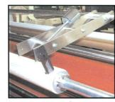
Unwind Slitting – is used to convert a wide roll of film on the unwind shaft to a smaller width web while laminating. The unused material remains on the roll core while the laminating material is introduced into the laminating
