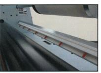
Static Elimination – When static build up from rolls of laminating film creates a hazard for operators; AGL has the solution. The AGL 6400 can be designed to add an optional pulsed DC static elimination bar designed to provide highly
