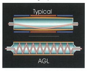
laminator between jobs saving valuable lamination film. Second, AGL uses a silicone coated steel roller construction without a crown. While our competitors use aluminum rollers and crown the silicone coating to compensate for their roller deflection (bending), we know this cost cutting technique will only cause you to have problems like in-feed waves (i.e.where the print buckles going into the laminator causing wrinkles and silvering). AGL rollers are guaranteed to have a
