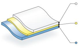
**Facestock:** 2 mil optically clear topcoated polyester features a minimum of 80% recycled polyester content. It offers excellent clarity and dimensional stability combined with good high temperature and humidity resistance. The optically clear polyester provides high resolution imaging with excellent
