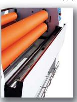
under the table or get on your knees (a laborious task on other laminators). The Easy Web Feed Table also features a dual latch for secure docking, yet has an elegant single handle release making it a smooth and fast one handed operation. Another not so obvious, but strong, feature on the Easy Web Feed Table is the hidden film guide. When the table is in the "disengaged position" it exposes the film guide ensuring that
