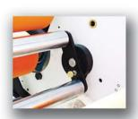
Cam you can run any film combinations you want. So stop trying to fight your print curl issues by using excessive brake tension that can cause post de-lamination. Stop running out (wasting) 5,10,15 feet of film just to get the film to lay flat. Start forming your film to the flat state your cus-
