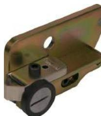
The V-Groove cutter enables the folding of Aluminum composite and PVC foamboard while cutting smoothly and silently without debris, noise or burred edges. The V-Groove removes exactly the correct amount from one side of the sheet material to allow a strong 90° fold.
