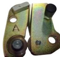
Cuts up to .040" (1mm) aluminum sheet material in a single pass. The cutting wheels are made of high-carbon hardened steel.
