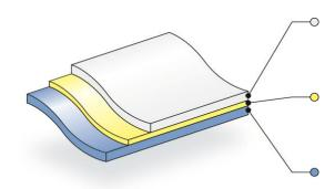
**Facestock:** 1.2 mil clear film with outstanding outdoor durability. Offering excellent dimensional stability combined with good solvent, elevated temperature, and UV resistance.
